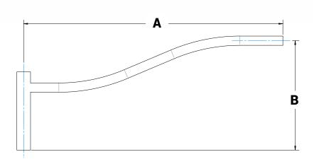
Architectural Arm 16 is constructed of extruded aluminum tubing. This mast arm integrates with poles or tenons of 3-1/2", 4", 4-1/2", or 5" OD and is secured with 3/8" stainless steel Allen set screws. Contact NLS for custom configuration or others mounting options. Arms are designed, tooled,
