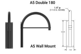
Architectural Arm 5 is constructed of extruded aluminum tubing. Integrates with poles or tenons of 3-1/2", 4", 4-1/2", or 5" OD and is secured with 3/8" stainless steel Allen set screws.
