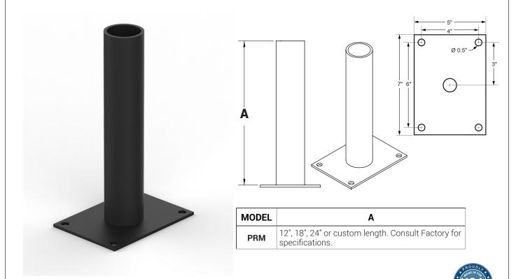
Pier Mount is constructed of extruded steel tubing. Integrates with poles or tenons of 2-3/8" or 3" OD. Contact NLS for custom configuration or others mounting options. Arms and Adapters are designed, tooled, fabricated and assembled in the USA.
